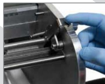
Three setting pressure bar for improved versatility. Can de-blister products up to 20mm in size. Desktop unit that includes handles for easy manoeuvrability.
