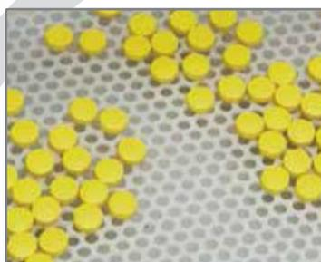
Mesh insert tray to catch de-blistered medication and allow foil fragments, dust and debris to fall through the holes reducing contamination.
