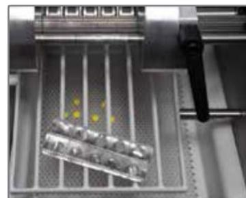
Unique foil catcher try to prevent contamination and allow operator to continually feed the machine. Can be positioned to allow discarded foils to fall into a bin.
